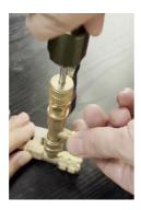
2.Lower the valve stem, rotate it slightly to engage with the valve core, then turn the handwheel counterclockwise to remove the valve core.
